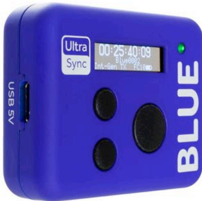
UltraSync BLUE is our first timecode sync product to use Bluetooth® pairing to connect and synchronise recording devices. Once connected, timecode and sync metadata is transmitted wirelessly from the UltraSync BLUE directly into the media file of connected devices.
