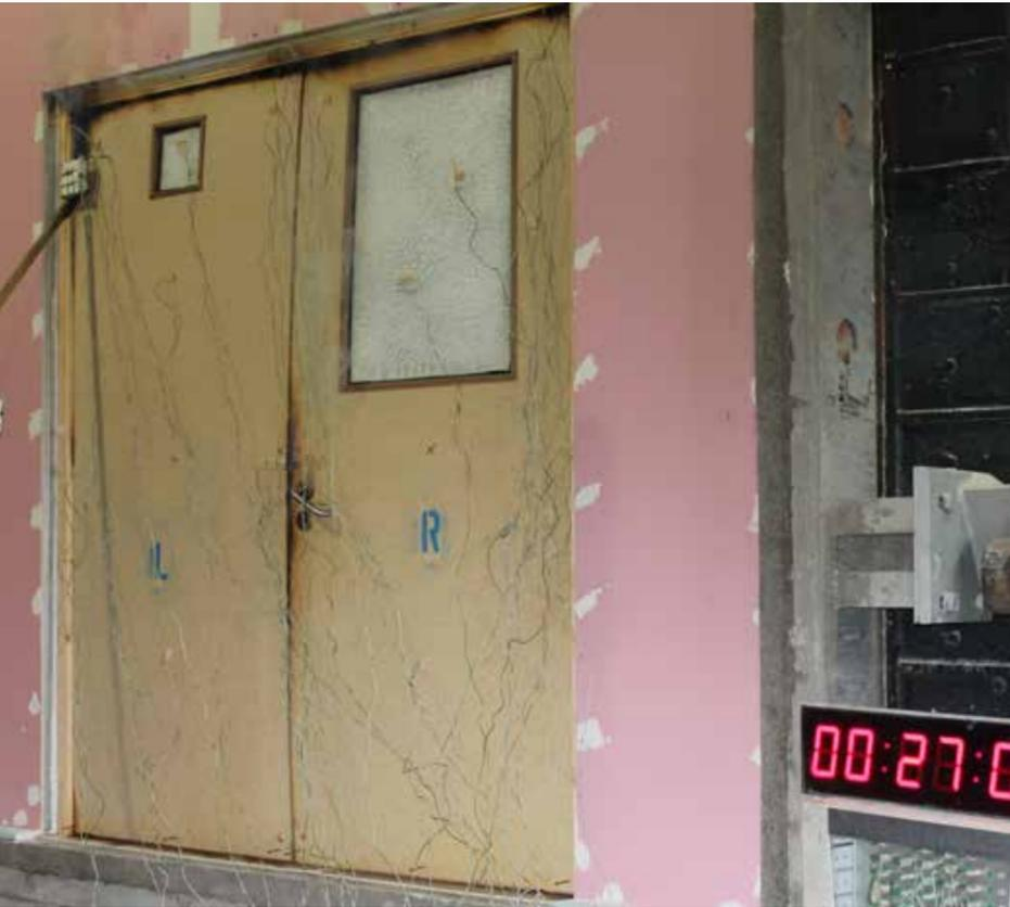
◀ A fire door undergoing independent testing.
